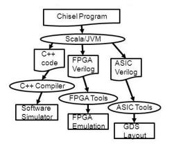
The generated code from chisel is compatible to be used by any standard ASIC or FPGA tools
